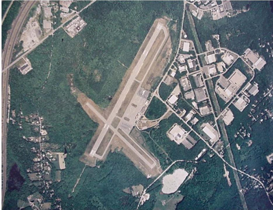
Built in 1951 and having a 5,000-foot primary runway and a 3,210-foot crosswind runway, SFZ is able to accommodate full operations by most small and mid-sized corporate jets, although larger aircraft (such as the Gulfstream G-IV) occasionally do operate there at reduced weights, due to the runway length constraints.
